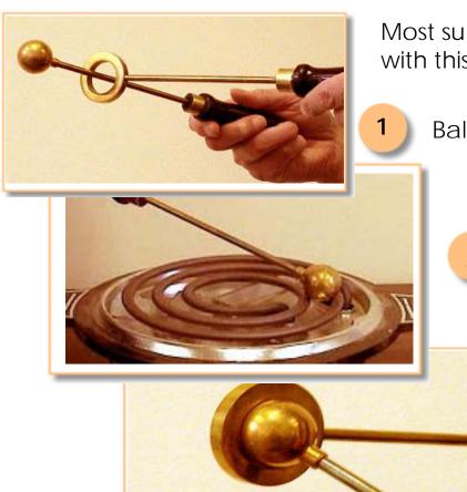
Most substances expand when heated, as shown with this metal ball and ring.
