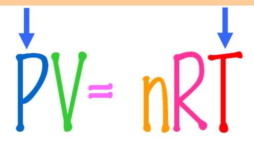
If we reduce the pressure and keep the volume constant, the temperature goes down.
