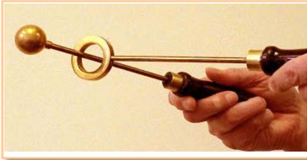
Most substances expand when heated, as shown with this metal ball and ring.
