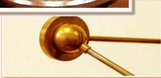
3 Heated ball has expanded, no longer goes through the ring.
